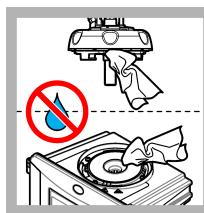
**16.** Make sure that there is no water on the process head (or the automatic cleaning module). Dry all possible spills to prevent water ingress on the vial compartment.
