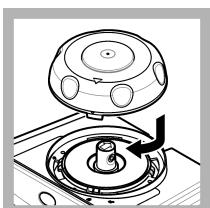
6. Install the calibration lid. Make sure that the calibration lid is in the closed position. Refer to [Installation](#) on page 3.
