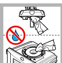
25. Make sure that there is no water on the process head (or the automatic cleaning module). Dry all possible spills to prevent water ingress on the vial compartment.
