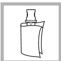
6. Clean and dry the verification standard vial with a no-lint cloth. Refer to [Prevent vial contamination](#) on page 16.
