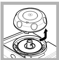
16. When the status indicator light flashes green, remove the calibration lid.
