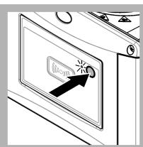
21. Push the button on the front of the instrument.
