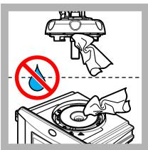
18. Make sure that there is no water on the process head (or the automatic cleaning module). Dry all possible spills to prevent water ingress on the vial compartment.
