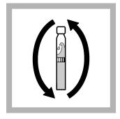
**1.** Invert a few times to bring the sediment into suspension.
