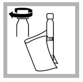
**3.** Close the cuvette, thoroughly clean the outside of the cuvette.
