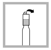
Carefully remove the foil from the screwed-on DosiCap Zip.
