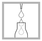
2. Pipet 0.5 mL Reagent B. Close Reagent B immediately after use.
