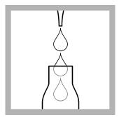
**10.** Pipet into the cooled cuvette: **0.5 mL Reagent B**. Close Reagent B immediately after use.
